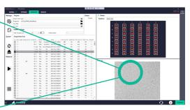
The measurement results are returned by the HORUS software. Each parameter is visible on a simple graphical interface with the possibility to follow up to 96 running cultures on user friendly charts.
